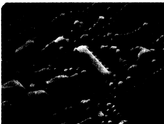
Figure 26. Electron micrograph of an \text{LaCrO}_3 ingot to which 7 mole % of calcium chromite has been added.
