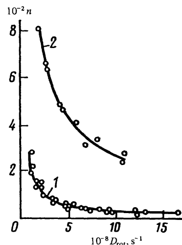
Figure 6. Influence of mobility of medium on ratio of times of translational and rotational diffusion ( \eta = \tau_{\text{rot}}/\tau_{\text{tr}} , with \tau_{\text{tr}} = x/2D_{\text{tr}} ( x = 5 \text{ \AA} ) and \tau_{\text{rot}} = 1/6D_{\text{rot}} , where x is the translational displacement of the probe, and D_{\text{tr}} and D_{\text{rot}} are the coefficients of translational and rotational diffusion) in rubbers at different temperatures: 1) polyenes; 2) polybutyl rubbers.
