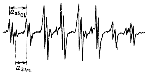
Figure 1. The EPR spectrum of the t -butyl- \alpha -chlorobenzynitroso-radical in benzene 49 .
