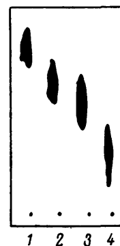
Figure 6. TLC of PMMA on silica gel in the 29:71 chloroform + methanol system. Molecular weight of PMMA M_w : 1) 4.3 \times 10^4 ; 2) 1.14 \times 10^5 ; 3) 1.65 \times 10^5 ; 4) 4.12 \times 10^5 .
