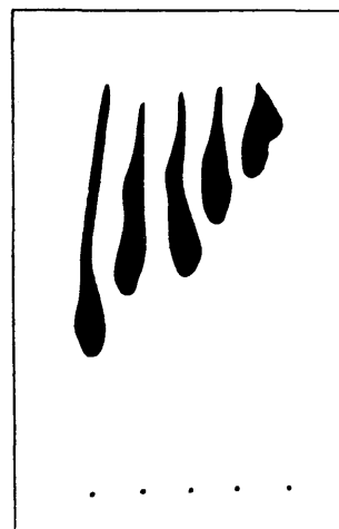
Figure 11. The "viscous" form of the chromatographic spot of PS with M_w = 8.7 \times 10^5 in TLC on KSK silica gel in benzene; 100, 40, 30, 20 and 10 \mu\text{g} of PS deposited from left to right.
