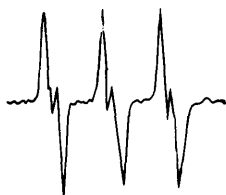
Figure 4. The EPR spectrum of the nitroso-radical obtained on ultraviolet irradiation of \text{CCl}_3\text{Br} in the presence of MNP. 47
